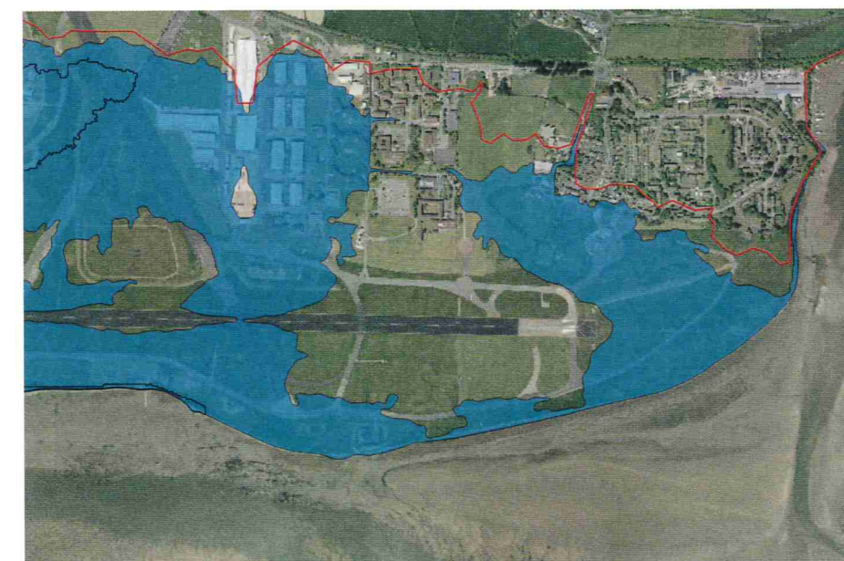
Figure 3 Aerial view of the Taw estuary in Devon showing existing flood boundary (light blue shading) and the projected future flood-level extent (red line) taking into account a 1 m sea-level rise
